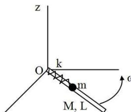
$$\text{SOL: } \begin{cases} \dot{r} = \frac{p_r}{m} & \dot{p}_r = \frac{m r p_\phi^2}{(m r^2 + I)^2} - k(r - l_0) \\ \dot{\phi} = \frac{p_\phi}{I + m r^2} & \dot{p}_\phi = 0 \end{cases}$$
