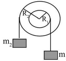
SOL:  $\ddot{\theta} = g \frac{m_2 R_2 - m_1 R_1}{m_1 R_1^2 + m_2 R_2^2}$
