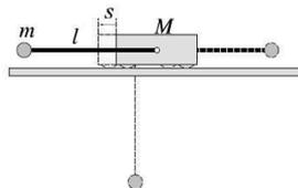
SOL: a)  $s = -\frac{2m}{M+m}l$ , b)  $v = \sqrt{\frac{2M}{M+m}gl}$ ,  $V = \frac{m}{M} \sqrt{\frac{2M}{M+m}gl}$
