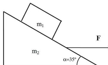
SOL:  $F_{min} = (m_1 + m_2)g \frac{\sin \alpha - \mu \cos \alpha}{\cos \alpha + \mu \sin \alpha} = 6.49\text{ N}$ ,  $F_{max} = (m_1 + m_2)g \frac{\sin \alpha + \mu \cos \alpha}{\cos \alpha - \mu \sin \alpha} = 6.49\text{ N}$
