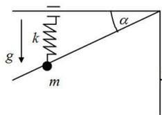
$$\text{SOL: } \ddot{r} + \left(\frac{k}{m} \sin^2 \alpha\right) r - \left(g + \frac{kl}{m}\right) \sin \alpha = 0, r = (r_0 - r_e) \cos(\omega t) + r_e,$$
